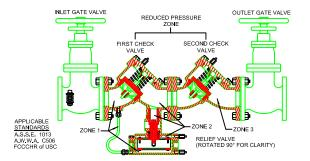
MASTER METER ASSEMBLY W/BY-PASS & REDUCED PRESSURE BACKFLOW PREVENTION ASSEMBLY (RPBA)
